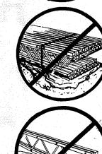
It is okay to stack the bundles as long as an adequate number of stickers are provided to prevent damage, and normal safety precautions are followed. During storage at the jobsite, joists should be given the same protection from weather as is normal with other wood products.
