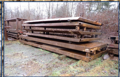
ASSORTED TRENCH BOXES
