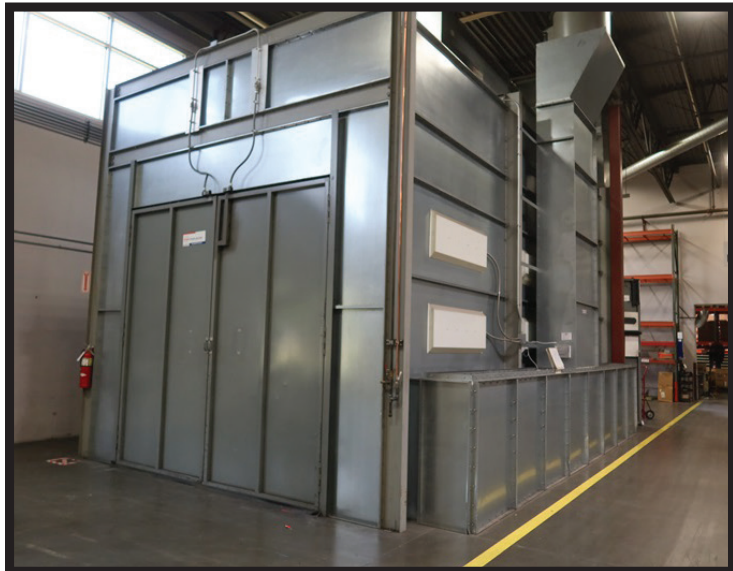
GLOBAL FINISHING SOLUTION SDG-1412PDT-26-S SIDE DRAFT DRIVE THRU SPRAY BOOTH
