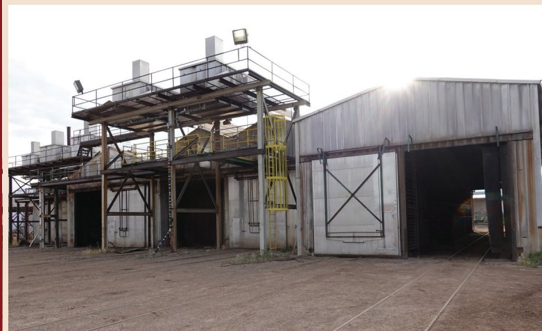
(6) STREAM FIRED ALUMINUM DOUBLE TRACK KILNS W/2022 KILN MANAGEMENT CONTROLS
