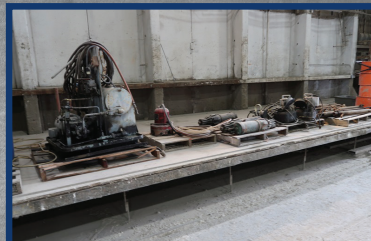
CONCRETE STRESS EQUIPMENT
