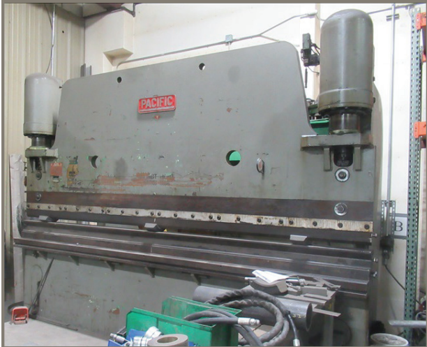
PACIFIC 200 12' 200 TON X 12' HYDRAULIC PRESS BRAKE, 36" THROAT, 14" WIDE, TOOL BED, CUSTOM DIE & STRAIGHTENING DIES
