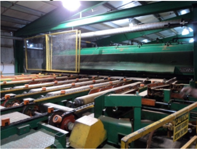
Newnes Optimized Trimmer TA-24-RH-156 with adjustable trim fence, 12 Smart gates for additional re-manning
