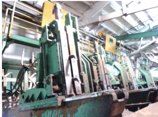
CME 24" Slant single cut headrig with 4 knee carriage, slabber head Inovec scanning optimization, Letson Burpee single Cut LH Bandmill
