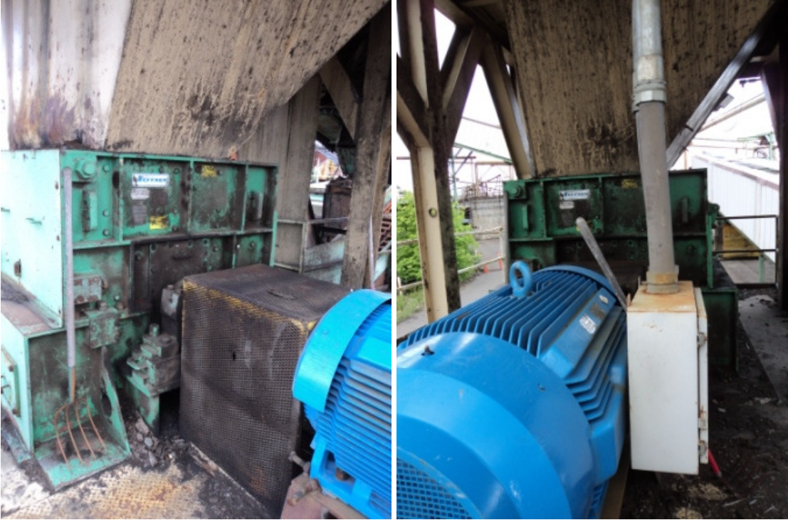
Jeffrey WB58 Hog, SN 11671 with 400 HP 1185, 460V Toshiba Motor
