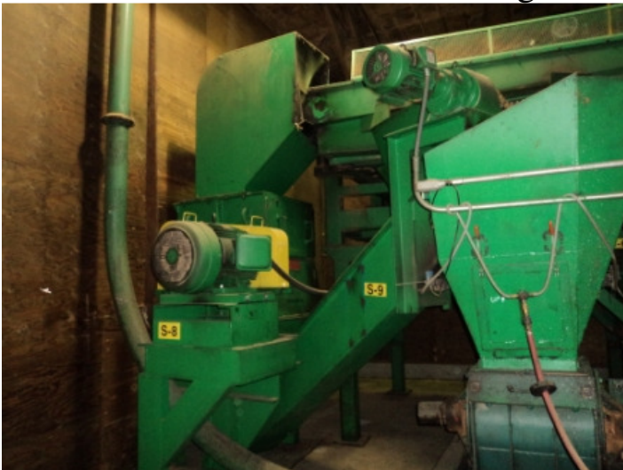
West Salem Machine 2420BR Hog with WSM HD8OD Shaker Screen
