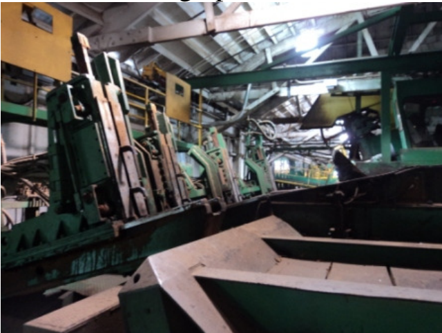
CME 24" Slant single cut headrig with 4 knee carriage, slabber head Inovec scanning optimization, Letson Burpee single Cut LH Bandmill
