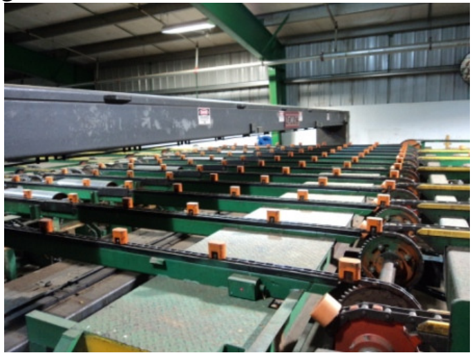
Newnes Optimized Trimmer TA-24-RH-156 with adjustable trim fence, 12 Smart gates for additional re-manning
