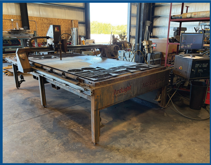
2021 ARCLIGHT DYNAMICS ARC MAX 5X10 CNC PLASMA CUTTING TABLE SYSTEM
