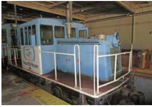
1943 GE EDM B-B-90/90-2GE733, 300 HP DIESEL ELECTRIC SWITCHING LOCOMOTIVE
