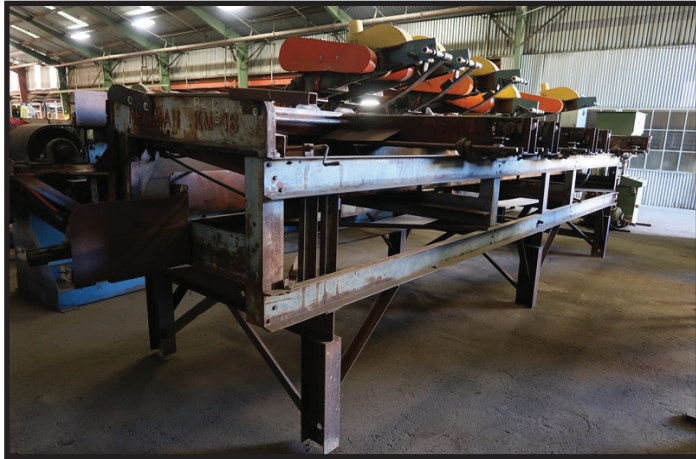
NEWMAN K16 MULTI-SAW 5-HEAD TRIMMER, 16' CAPACITY, 7-1/2 HP MOTORS, 4' 5-STRAND FEED THRU TRANSFER, OUTFEED & CHAIN BELT, GEARHEAD MOTORS
